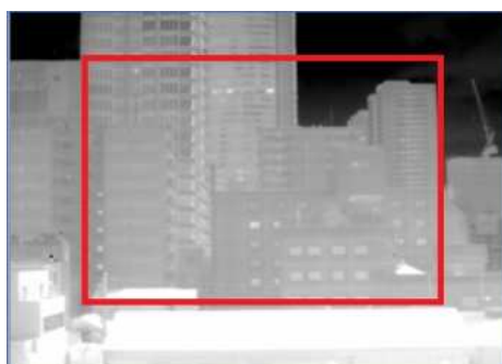
Image of element pitch 17 \mu m camera
